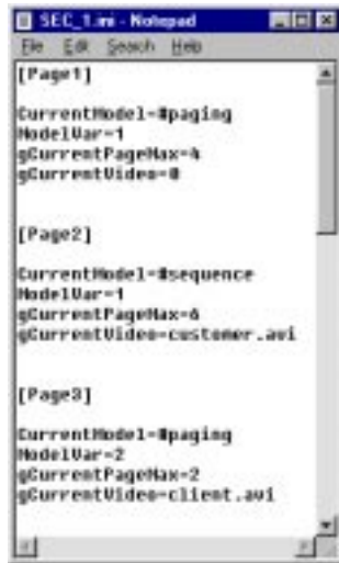
Figure 2. (Right) This text "ini file" contained all the details for each page in the project—and could be edited from outside the source Director file.
